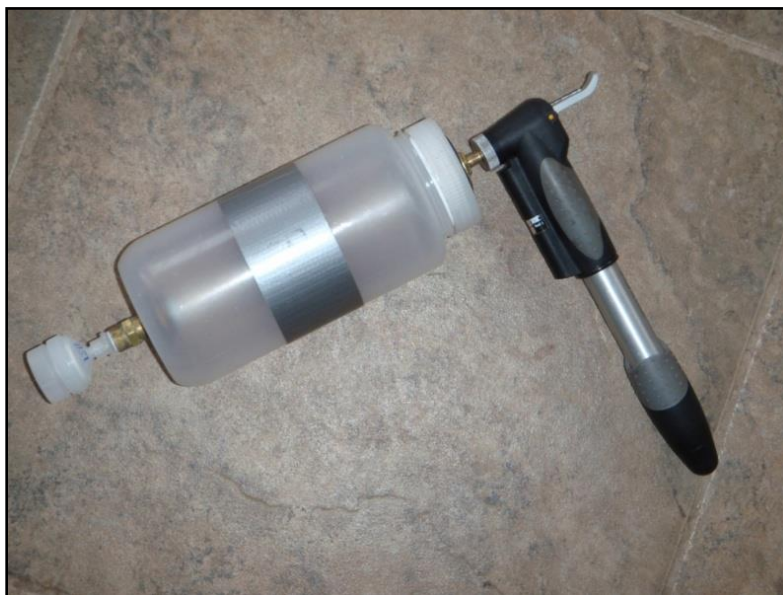
Figure 1. A bike pump connected to the modified Nalgene bottle and filter medium used in collection of eDNA samples, following the Pisces Molecular protocol.
